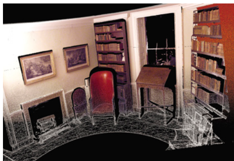
Computer scientists at Carolina and the University of Virginia are creating a model of Thomas Jefferson's Monticello. Using a laser-range scanner, millions of data points can be gathered quickly and precisely and transformed into highly accurate three-dimensional models for study. The scanner used in this project is marketed through a startup venture from 3rdTech, which links university inventions with the marketplace.
